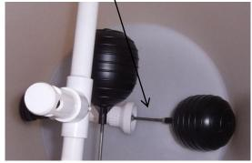
The Check Valve MUST close when the float is in the down position. The 2 floats may touch. It is not necessary to cement the parts together, but may be done if preferred.
