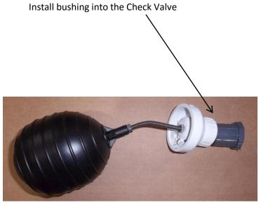
Install check valve/bushing and float onto pipe nipple with the rod in the bent up position. The Check Valve MUST close when the float is in the down position. The 2 floats may touch. It is not necessary to cement the parts together, but may be done if preferred.
