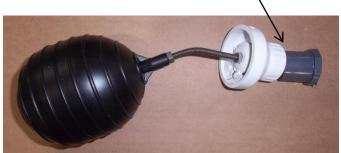
Install check valve/bushing and float onto pipe nipple with the rod in the bent up position. The Check Valve MUST close when the float is in the down position. The 2 floats may touch. It is not necessary to cement the parts together, but may be done if preferred.
